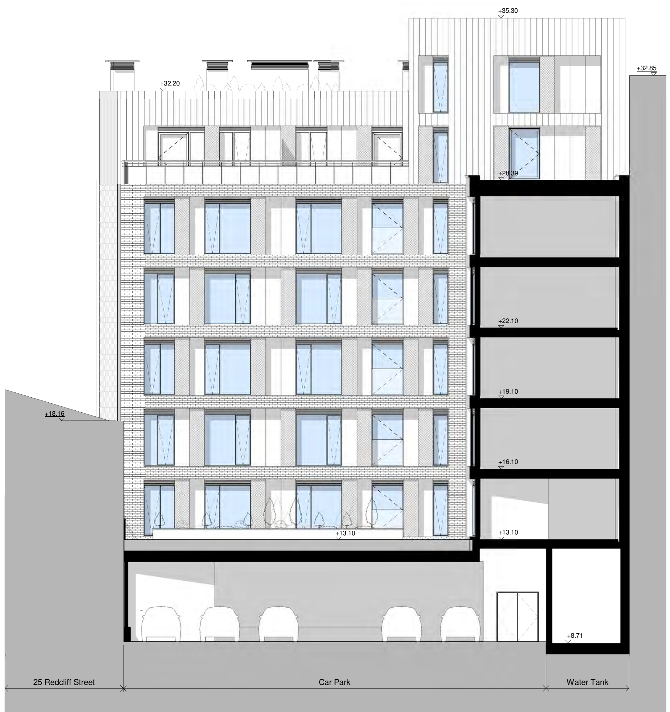
3 BLOCK A - AMENITY SPACE 1 - EAST ELEVATION 1:100
